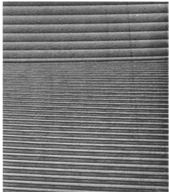
Figure 3 An etched (211) surface of InSb single crystal (doped with Te) cut along the growth axis exhibiting rotational impurity heterogeneities. The upper part was pulled with rotation in the absence of a magnetic field; the lower part was pulled in a transverse magnetic field of 4000 gauss. Note the adverse effects of the applied field on the homogeneity of dopant distribution ( \times 200 ).
